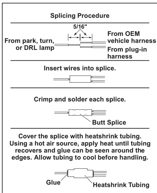
**NOTE: Avoid using an excessive amount of solder, as it can result in wicking. Wicking occurs when solder travels up the wire core. This may cause the wire to become stiff or brittle, which could lead to a broken or open circuit.**
