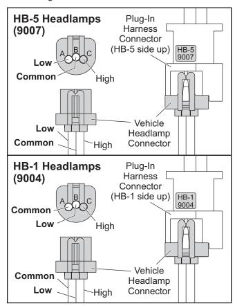
For vehicles using the 29050 Harness Kit with the 26641-1 or 28860-1 Adapter Kit: Plug the adapters into the plug-in harness with the locking tabs on the same side as the "HB-5" text.
