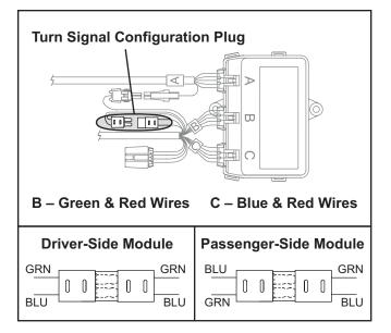
Connect the single-wire connector from the vehicle lighting harness to the single-wire connector from the plug-in harness.
