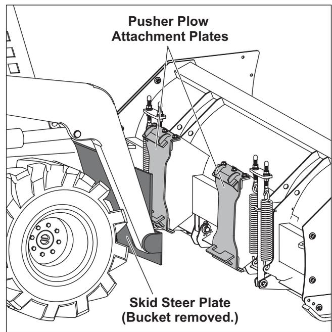
3. Tilt the skid steer plate forward and position the top edge of the plate under the receiving pockets on the attachment plates.
