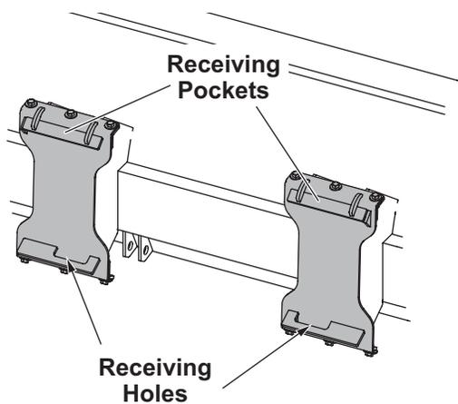
4. Slowly raise the arms on the skid steer and tilt the skid steer plate toward the cab until the snowplow mount plates are flush with the skid steer plate. Turn the skid steer engine OFF.
