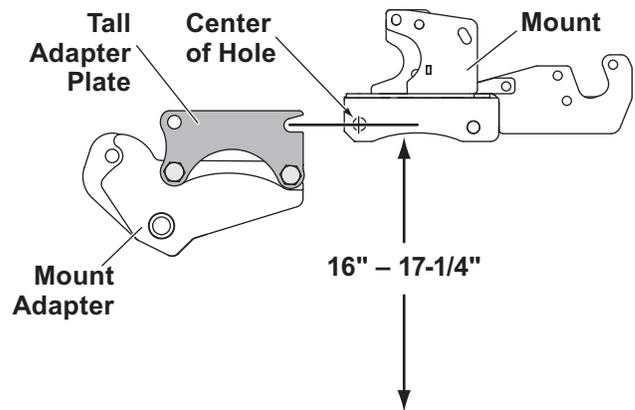
5. Position the adapter plate against the driver's side portion of the mount adapter as shown. Insert a 3/4" x 2-3/4" cap screw through the lower front adapter plate hole and through the appropriate hole on the mount adapter. Secure with a locknut.
