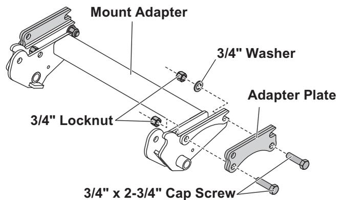
6. Insert a cap screw through the rear adapter plate hole, through the slot on the mount adapter and through a washer. Secure with a locknut.
