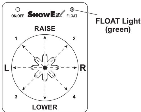
From the center position, the control lever can be moved in one of eight directions to control various movements of the snowplow blade. To change from one movement of the blade to another, the control lever must be moved back to the center position before selecting the desired function. Whenever the lever is released, it should spring back into the center position to stop any blade movement.
