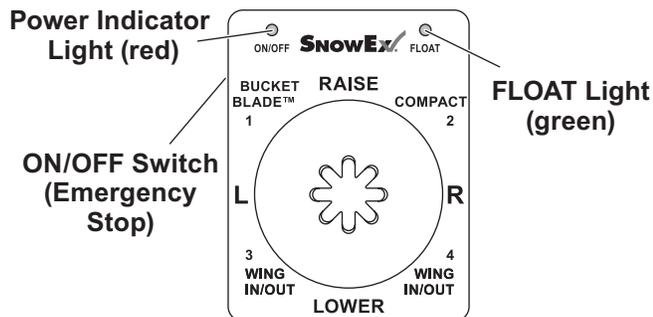
**SECURITY GUARD™ system enabled controls have numbers 1 through 4 on the faceplate.**
