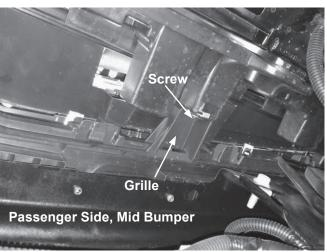
4. Remove the two bumper cover screws located on the inside of each front wheel well. If the vehicle is equipped with fender trim, it will need to be displaced in order to access the screws.
