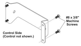
3. Install the control side of the bracket to the control using four #8 x 3/8" Phillips head machine screws.
