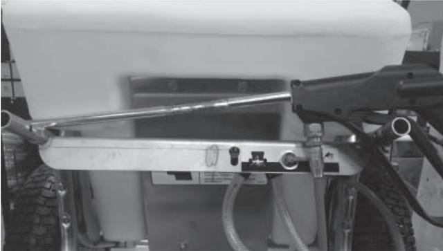
2. Install the handle assembly to the tank base assembly using the provided 5/16" cap screws and nylon locknuts.
