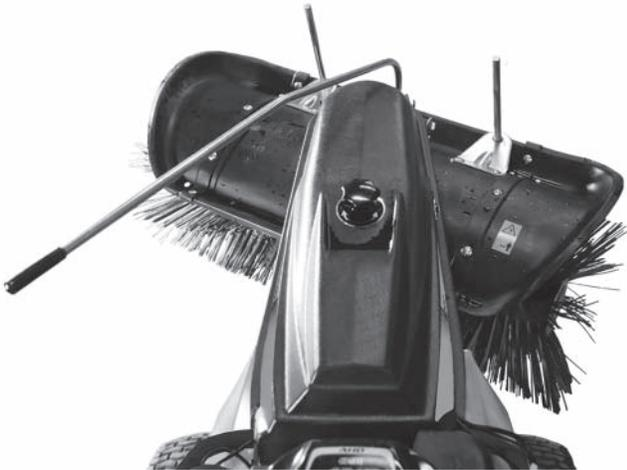
A sideways setting is recommended if using the optional debris collector. This will allow sweeping against a wall or curb. (Debris collector box is an optional accessory).
