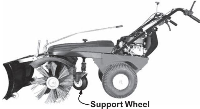
The adjustment knob is located above the support wheel.
