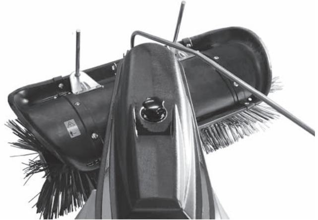
If you use a plow, an angled direction must be used. Shown below: Ejection to the left.
