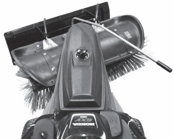
To adjust brush angle: Lift the lever; Turn the brush in the desired direction; Release the lever and ensure the lever is latched in place.
