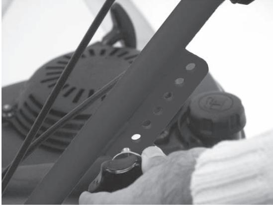
Loosen the knob on both sides and choose the desired position
