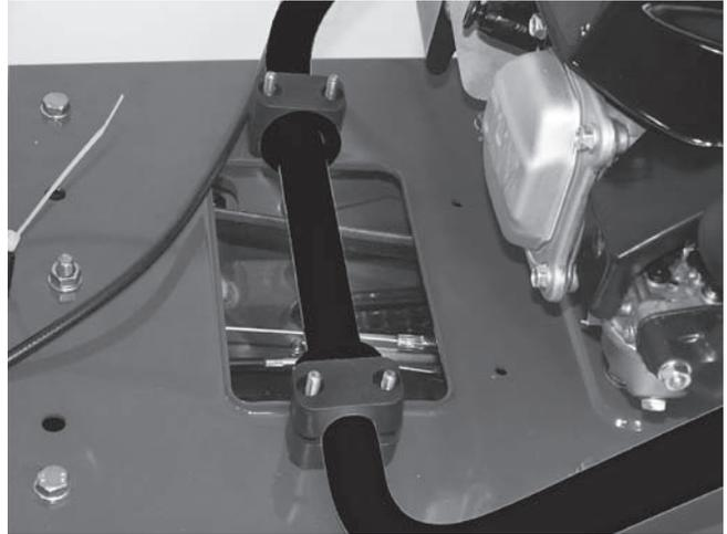
4. Put fixing plates on the studs. Position as shown.
