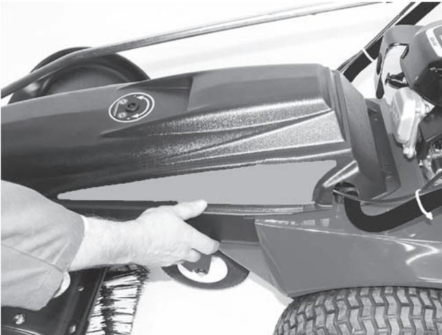
14. Put TORX® screws with the countersink washers through the mounting holes on the cover and thread into the snap nuts.
