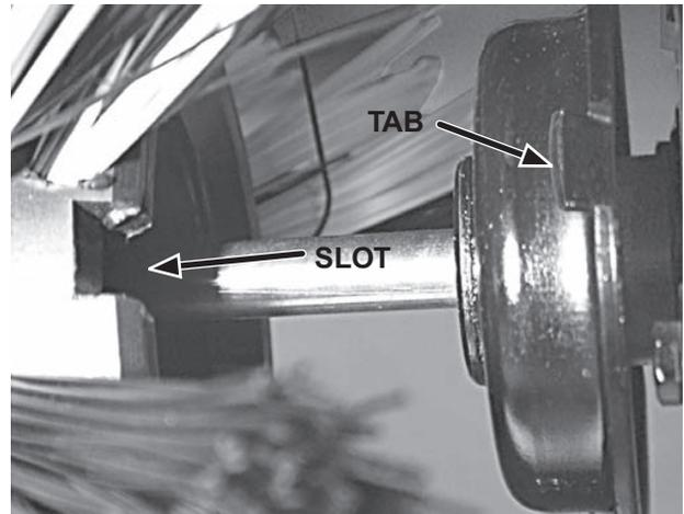
7. Put the left brush on. Make sure the brush is locked onto center cap-gear.
