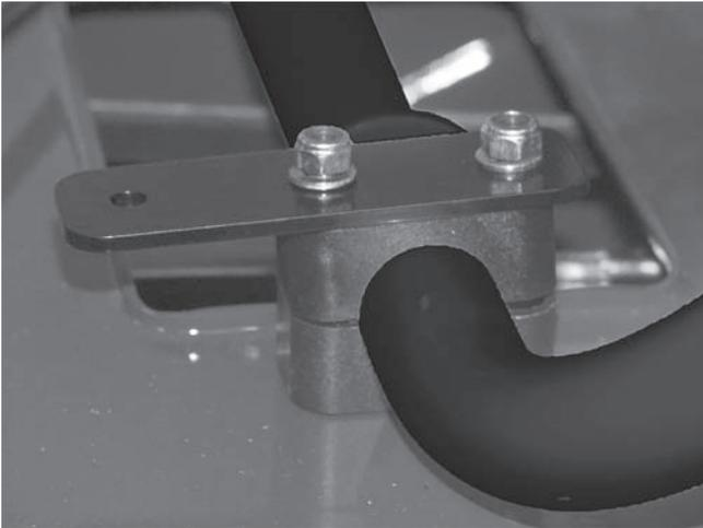
6. Using a 10 mm wrench, tighten the nuts so the handlebars will still move, but not fall.
