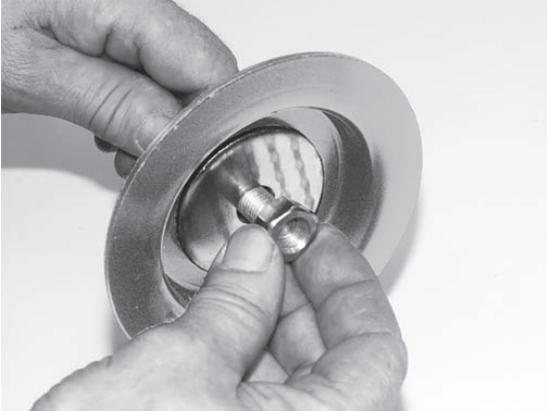
3. Tighten nuts to hold the cap and washer in place.
