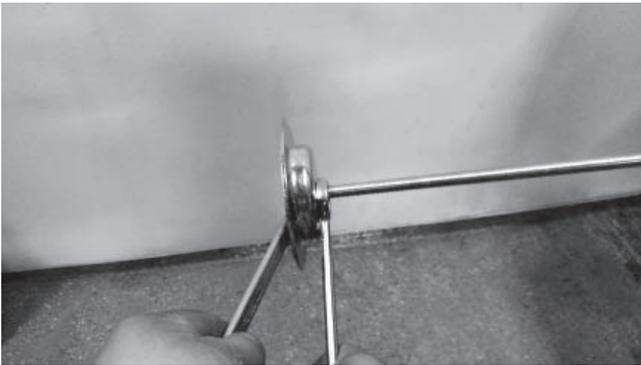
4. Put the axle with the cap, washer and right brush through the drive source (centered underneath the brush cover).
