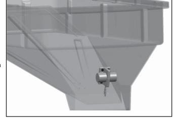
Step 4: Install an inline 10 amp. fuse on the positive (red) lead from the battery to the switch. Locate an easily accessible place, out of the elements, for the fuse and remove approx. 3" of the black outer jacket exposing two single leads (red and black). Cut the red lead in half and strip a 1/4" off each lead. Insert into the fuse connector and crimp. Insert 10 amp. blade fuse into connector.
