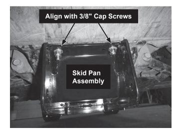
Place the U-bolt shim plates in position on the top side of the skid pan assembly. Position two U-bolts on each side of the mount (four total), as shown. Check that the U-bolts have at least 1/4" clearance from any other vehicle components. Adjust the position forward or aft, as needed. Secure with 3/8" washers and 3/8" locknuts.
