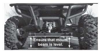
Measure the distance between the mount beam rear hole and the ground. If it exceeds 11-1/2", install the accessory Height Adapter Plate Kit (PN 77555) to ensure optimum plowing performance.
