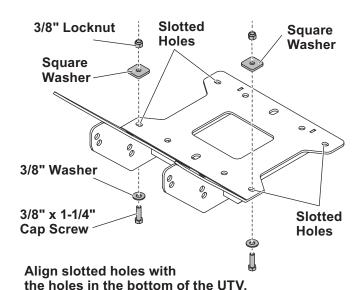
4. Secure the rear of the skid pan assembly to the UTV using 3/8" x 1-1/4" cap screws, 3/8" washers on top of the UTV skid plate and on the bottom of the skid pan assembly, and 3/8" locknuts.
