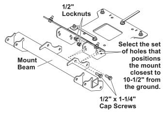
10. Ensure that the mount beam is level with the ground and tighten the mount beam fasteners according to the torque chart.
