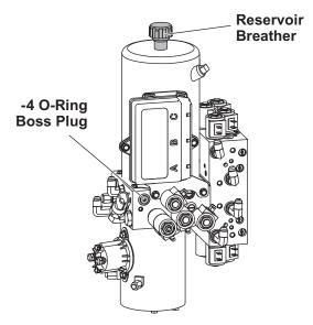
Install the pressure switch in place of the O-ring boss plug. Gripping the hex portion only, tighten the pressure switch to 10–13 ft-lb.
