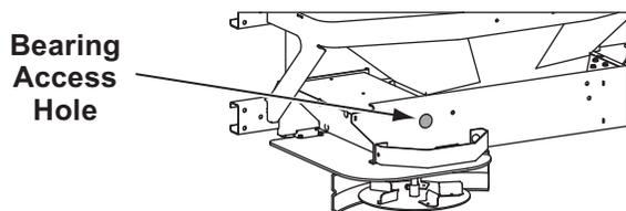
**Model SP-1575:** Access the auger bearing grease zerk from the tailgate side of the spreader frame. (To add an access hole and plug to an SP-1575 frame, order service kit 76711.)
