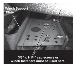
6. If a winch is not being installed, insert 3/8" x 1-1/4" cap screws through the indicated holes in the winch plate and through the holes in the forward frame cross member. Secure with 3/8" locknuts.
