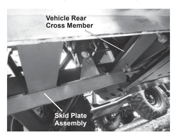
5. Position the winch plate as shown below and install to the winch support plate and skid plate assembly using 3/8" x 1-1/4" cap screws and 3/8" locknuts in four places. Tighten all fasteners according to the torque chart.
