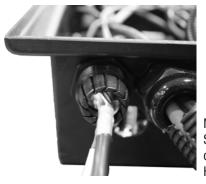
Note: it is optional to remove the Spinner Harness for the installation. It only makes it easier to tighten the PWX Harness Cord Restraint.
