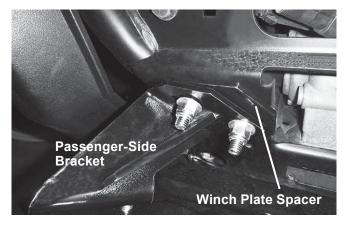
If the vehicle is equipped with a winch: Align one hole in the winch plate spacer with the bottom hole of the passenger-side bracket to fill the existing gap. Install the bracket and spacer using two  $3/8" \times 1-1/2"$  carriage bolts and 3/8" locknuts. (The second hole in the spacer is not used.)
