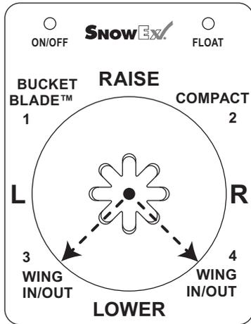
**NOTE:** If a control function times out before the desired blade movement is complete, release the lever to the center position, then move it back into the desired function.
