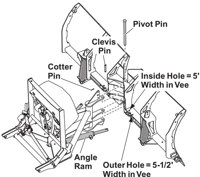
Install a 1/2" x 2-7/8" clevis pin or 1/2" x 4" Grade 8 bolt (provided in the parts bag) from the top down to attach each rod. Secure the clevis pins with 5/32" x 1-1/2" cotter pins, and secure the cap screws with 1/2" locknuts.
