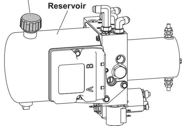
3. Check the fluid level in the reservoir. The fluid level should be 1-1/2" to 2" below the top of the reservoir. Add the recommended hydraulic fluid, if necessary. Do not overfill.
