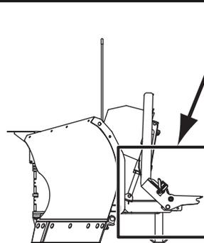
5. Move the hitch pin handle into the handle lock notch.
