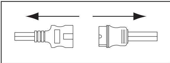
**NOTE:** After each disconnection of the snowplow, reapply dielectric grease to the electrical plugs to maintain the protective coating on the terminals.
