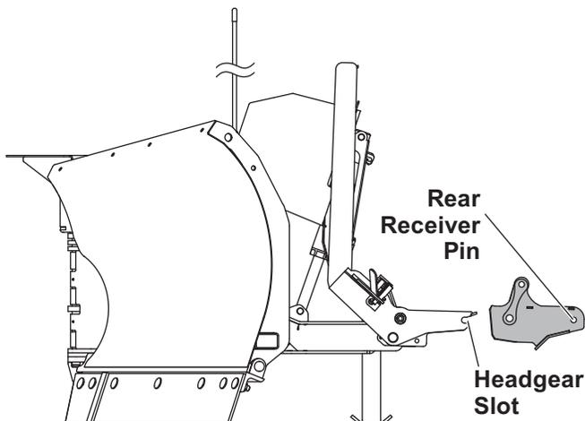
2. Hold down the lock lever and move the hitch pin handle out of the handle lock notch, allowing the spring to move the hitch pin handle forward.
