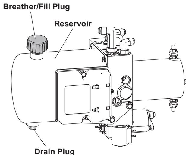
4. Remove the drain plug.
