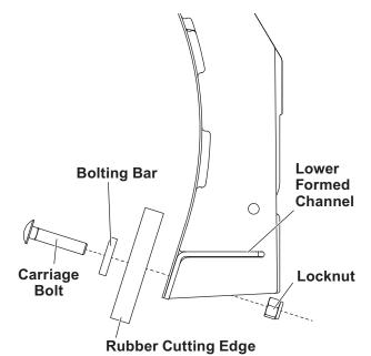
5. Adjust the position of the rubber cutting edge so that it extends approximately 1-3/8" beyond the bottom of the blade lower formed channel as shown. Tighten all the carriage bolts until the rubber starts to bulge.
