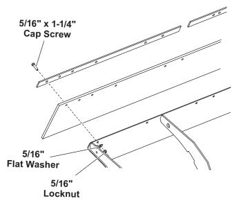
3. On 6'8", 8', and 8'6" blades, the deflector extends beyond the ends of the blade. Trim excess length from both ends of deflector and retainer bars as shown.
