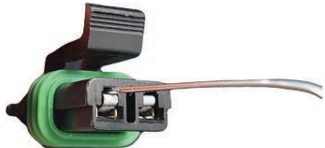
6. Gently pull the red wire out of the connector body. It should come free with ease, so if it isn't you may need to reposition the extraction tool to ensure the terminal lock tab is released. Damage may occur if excessive force is used.
