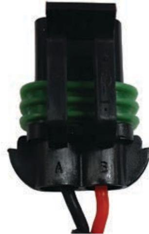
5. Insert terminal extraction tool or paperclip into the connector body as shown to a depth of about 5/16" to release the terminal lock on the red wire.
