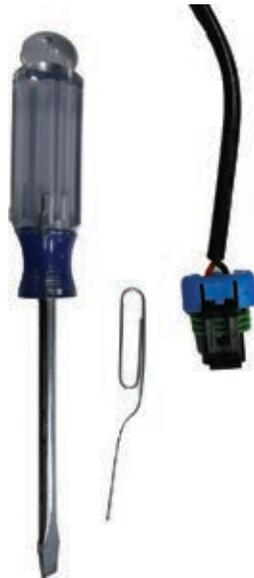
3. Gently pry secondary lock away from each side of connector body and set it aside for reuse.
