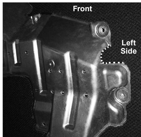
**NOTE: After five to ten hours of snowplow usage, retorque all mount assembly fasteners.**
