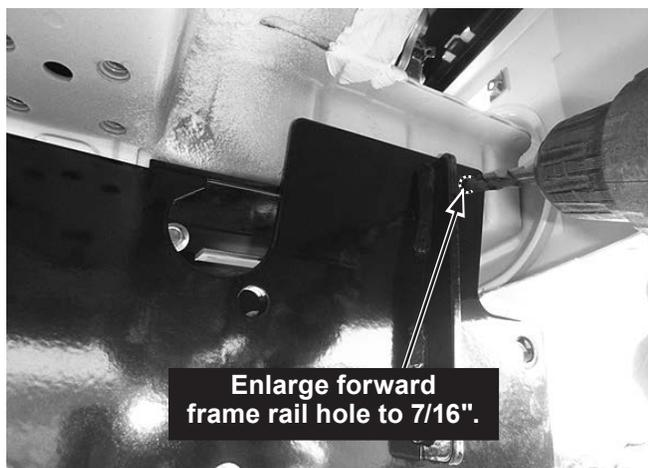
Place a 3/8" washer on each of two handled 3/8" x 1-1/4" cap screws. Install the fasteners through the enlarged brush guard holes. Secure with 3/8" washers and 3/8" locknuts. Hand tighten.
