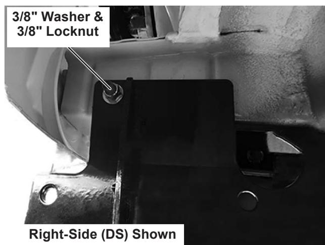
9. Install the mount beam as shown.
