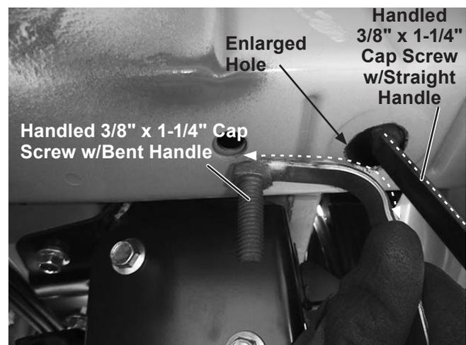
5. Bend the handles on two handled 3/8" x 1-1/4" cap screws as shown below. Insert the cap screw through the next access hole rearward and down through the bottom frame hole shown. Repeat for the other frame rail.
