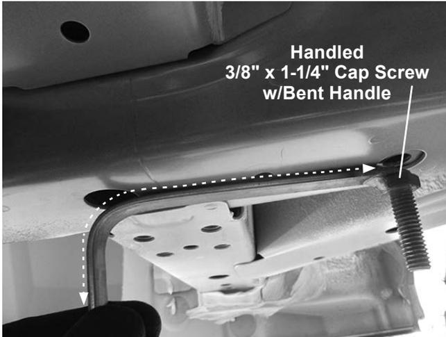
6. Position the right (driver's side) mount bracket against the bottom of the frame rail as shown. Ensure that the previously inserted handled 3/8" x 1-1/4" cap screws protrude through the mount holes as shown. Secure each cap screw with a 3/8" washer and 3/8" locknut. Repeat on the left (passenger's) side of the vehicle. Tighten the locknuts enough to ensure full contact of the mount to the bottom of the frame. Cut or bend excess handle length as needed to clear components in subsequent steps.
