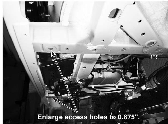
3. Insert a handled 3/8" x 1-1/4" cap screw through each of the holes enlarged in Step 2.
