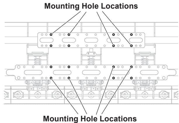
2. Install each attachment plate to the indicated holes with a 3/4" x 3" cap screw, 3/4" washer, and 3/4" locknut as shown. The notches in the attachment plates must face the center of the snowplow. Tighten to 269 ft-lb (365 N·m).
