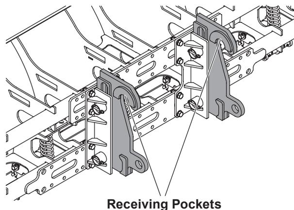
3. Slowly raise the arms on the loader and tilt the loader plate toward the cab until the mount plates are flush with the OEM attachment bracket.
