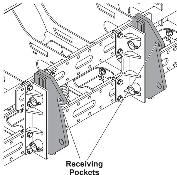
3. Slowly raise the arms on the loader and tilt the loader plate toward the cab until the mount plates are flush with the OEM coupler.
