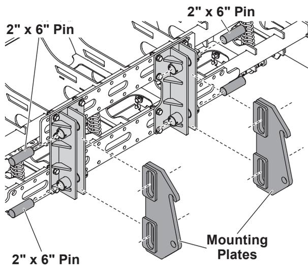
4. Secure each end of each pin with the eight provided 3/8" x 3" cap screws and 3/8" locknuts as shown. Tighten to 30.8 ft-lb (41.8 N·m).
