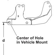
3. Use distance "d" from Step 1 and the following chart to determine the proper T-frame hole.
