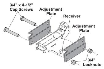
Insert a cap screw through the rear adjustment plate hole, through the slot on the receiver. Secure with a locknut.
