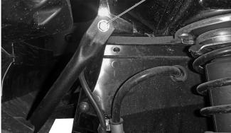
3. Remove and retain the four bolts from the front frame plate.
