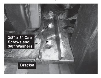
3. Slide a bracket assembly over the 3/8" fasteners protruding through the bottom of the winch mount plate. Fasten the bracket assembly to the winch mount plate using 3/8" washers and 3/8" locknuts as shown. Hand tighten the fasteners.
