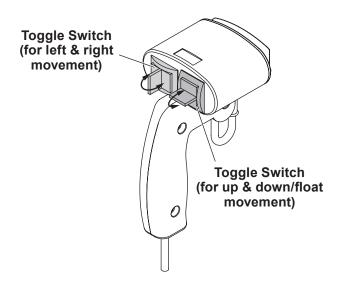
**Handle Grip Options:** The handle grip on the control can be positioned three ways – left-aligned, right-aligned, or in the center position.
