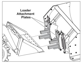
2. The bucket edge will rest against the attachment plates. The upper posts will fit inside the bucket and should be centered. The lower posts will be positioned under the bucket.
