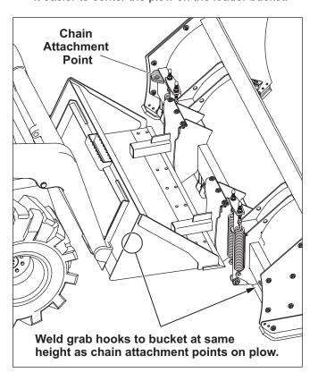
Use a supplied clevis attachment to connect one
