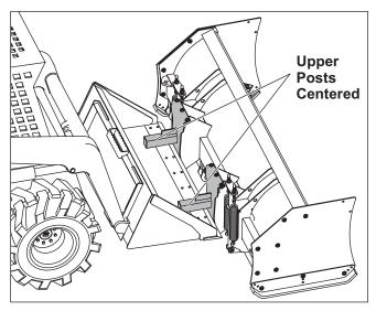
3. Attach the chains and ratchet binder to secure the plow to the bucket, as described in the next section.
