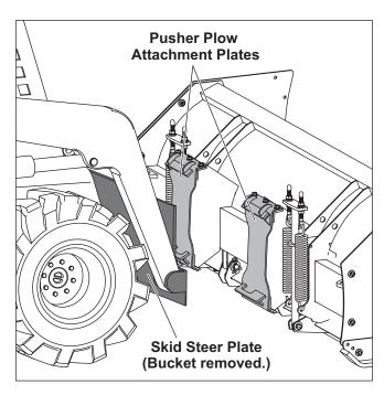
3. Tilt the skid steer plate forward and position the top edge of the plate under the receiving pockets on the attachment plates.
