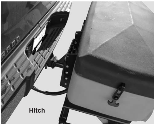
Receiver Adapter w/ Precision Pro 1675 spreader installed on truck.
