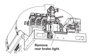
2. Install the hitch bracket to the pump platform using the 1/2" hardware provided.
