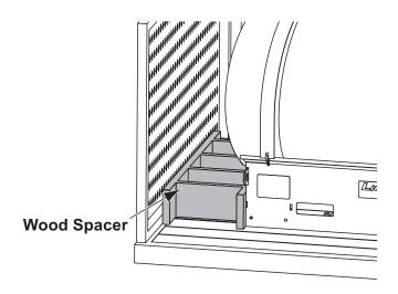
Failure to install a spacer could result in damage to the sprayer or vehicle.
