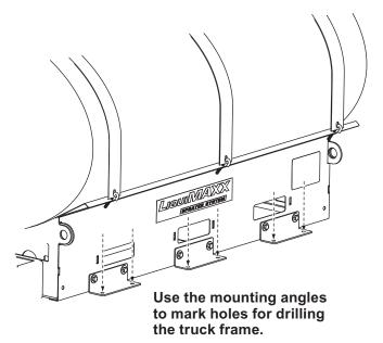
NOTE: Pay special attention when drilling or clamping dissimilar metals to aluminum bodies. Galvanic corrosion can occur if not handled properly. Contact vehicle manufacturer for recommended attachment practices.
