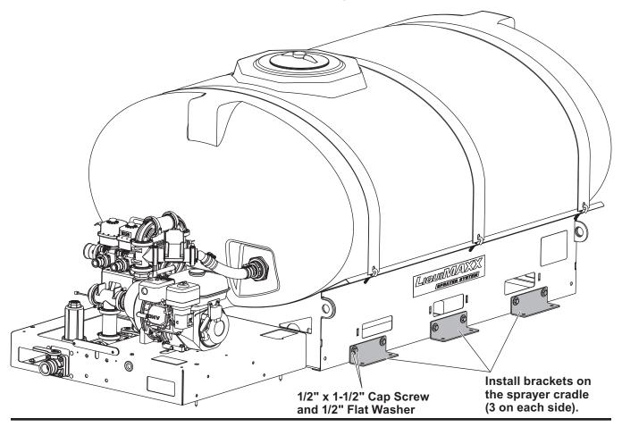
Install the sprayer in the truck bed against the spacer as described in the Installations Instructions for the Liqui Maxx™ sprayer system.
